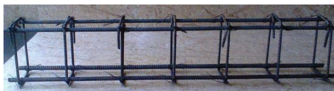
Fig. 4 Reinforcement cage - beams in flexure
