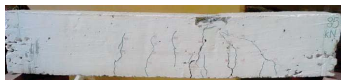
Fig. 10 Crack pattern of CB-F
