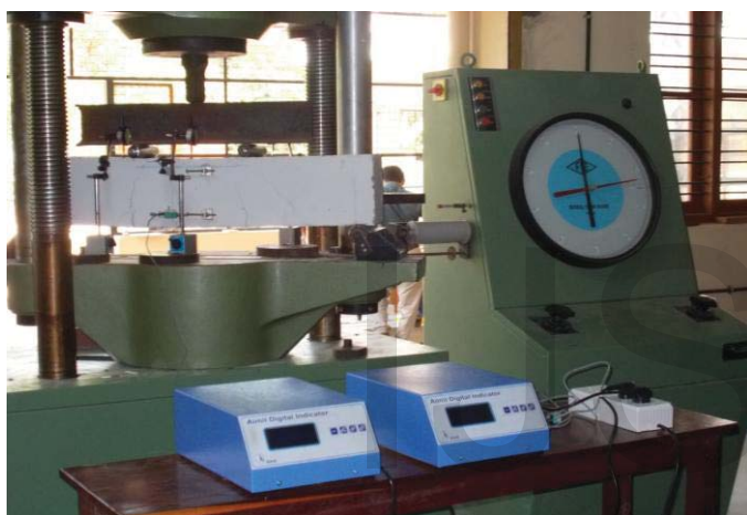
Fig. 8 Test set up of beams in Universal Compression Testing Machine(UTM)
