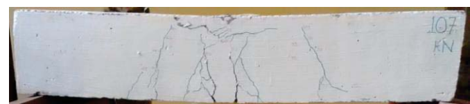
Fig. 11 Crack pattern of MKHB-F
